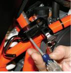
**8.** Attach the plastic cover using the two small Phillips screws.
