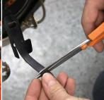
**3.** Trim the end of the rubber protector to the correct length with scissors.
