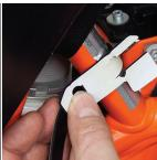
**2.** Place the rubber protector around the tube to determine the correct length required.
