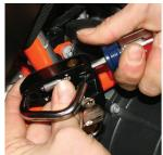
7. Place in desired location holding the top of clamp in place and pushing the open end of the clamp into the threaded end. Tighten the hose clamp using a #2 straight slot screw driver.
