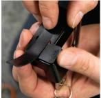
**4.** Remove the paper backing and attach the rubber protector to the back of the helmet lock.
