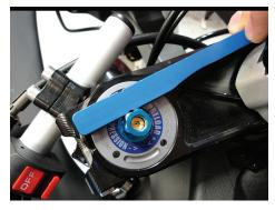
Next, align the notch on the end of the main arm with the center of the fork tube that is opposite from the handlebar you are measuring. Once the main arm is in this location, do not allow it to move through the next step.
