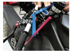
If you place the tool, and there is a space between the indicating rod and the handlebar, that means the handlebar is too far forward. Make adjustments to that handlebar, and check again with the tool. Move the tool to each side several times, and make adjustments as necessary to the sweep of the handlebars.
