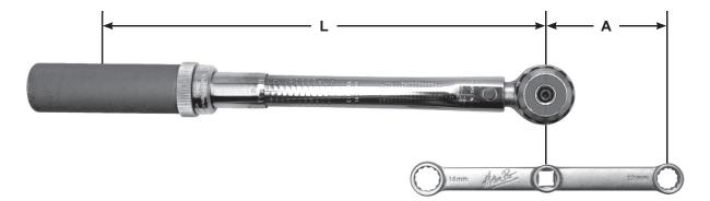
**NOTE:** When using 3 inches for distance "A", torque wrench and torque adapter must be in line. If the adapter is positioned at an angle to the torque wrench, distance "A" will be decreased. When the adapter is at a 90-degree angle to the torque wrench, distance "A" will be equal to zero (0).
