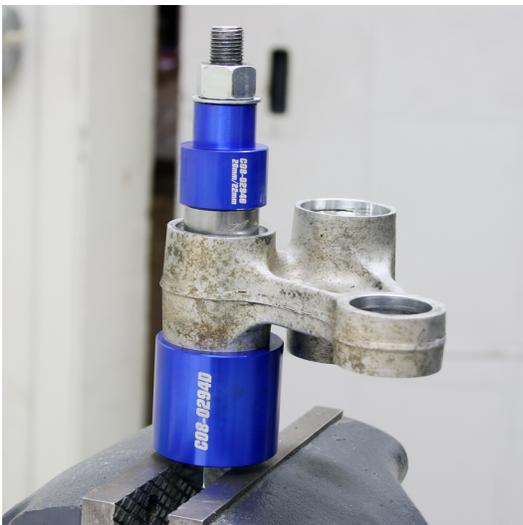
**e.** Install bearing onto the corresponding bearing driver as shown in Fig 6. The bearing driver will hold the loose needles in place during installation.
