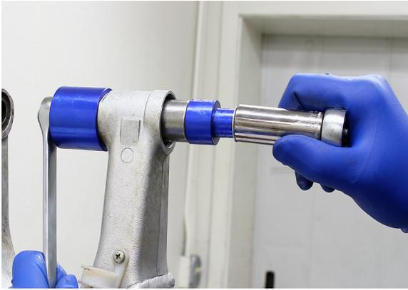
**g.** Assemble the bearing driver as shown in Fig 4. Tighten screw until the driver bottoms out on the inside bearing surface.
