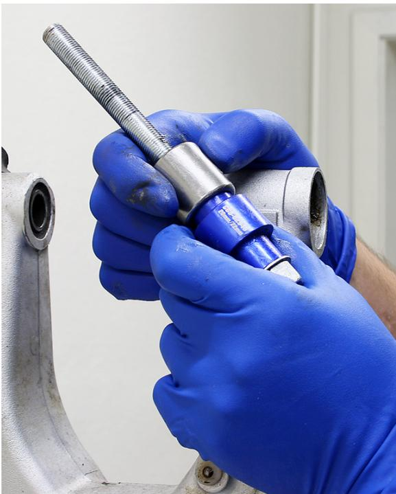
d. Clean all bearing surfaces and inspect for damage.
