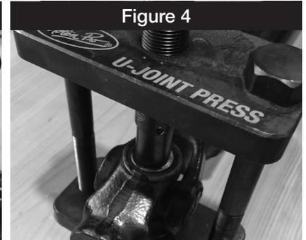
**Note:** This tool is designed to be used as both a punch and a press. If the U-Joint is stuck or requires a lot of effort on the main screw, use a brass hammer and strike the top of the main screw to jar the U-Joint loose. **MAKE SURE YOU REMOVED ALL THE CLIPS!!!!**
