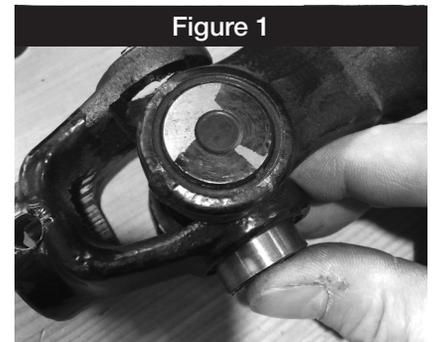
**2:** Flip the assembly over and install the second cup. Press the cup in until you can see the clip ring is exposed and install the clip. Carefully inspect the position of all the cups and that all of the clips are completely seated. Move the U-Joint through its range of motion to make sure everything is assembled correctly. Reinstall into the vehicle according to the service manual.
