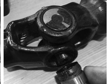
**5:** Repeat this procedure on the other side and remove the yoke from the U-Joint.
