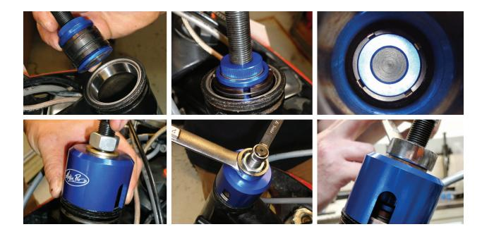
For installing the new bearing we recommend the Motion Pro Steering Head Race Driver (P/N 08-0550). To remove and replace the bearing from the steering stem we recommend the Motion Pro Steering Stem Bearing Tool (P/N 08-0544).
